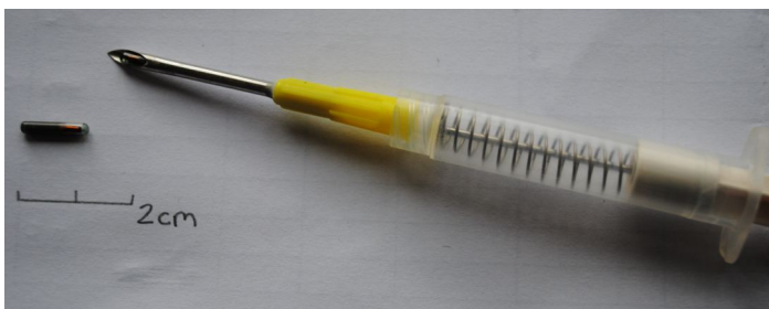
Illustration 8: PIT tag and injector.
