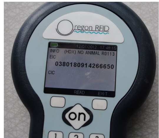
Illustration 7: 16-digit identity number of a tag on the portable reader.
