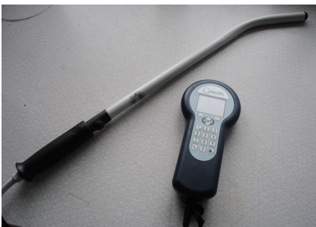
Illustration 6: Oregon RFID portable reader extended with stick antenna.
